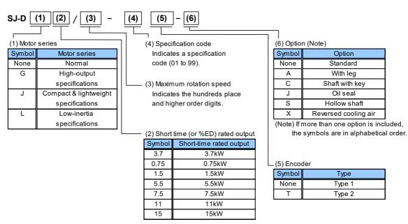
(Note) This explains the model name system of spindle motors, but does not mean all the combinations are available.
