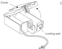
Open the cover while pushing the locking part.
