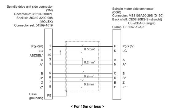
Spindle drive unit side connector Spindle motor side connector (DDK) Receptacle: 36210-0100PL Connector: MS3106A20-29S (D190) Shell kit: 36310-3200-008 Back shell: CE02-20BS-S (straight) (MOLEX) CE-20BA-S (angle) Connector set: 54599-1019 Clamp: CE3057-12A-3 0.5mm<sup>2</sup> Н P5(+5V) P5(+5V)  $0.5 \text{mm}^2$ 2 Κ LG LG 10 ABZSEL\* 3 Α 0.2mm<sup>2</sup> 4 A\* Ν A<sup>3</sup> 5 С В В 0.2mm<sup>2</sup> 6 R В\* В\* 7 В Ζ Ζ 0.2mm<sup>2</sup> 7\* 8 Ρ **Z**\*
