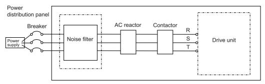
(Note) The noise filter must be prepared by the user.
