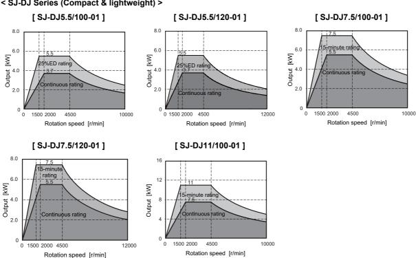
Actual acceleration/deceleration output is 1.2-fold of "Standard output during acceleration/deceleration" or (Note) "Short time rated output".
