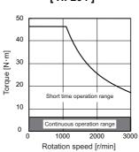
(Note) The above graphs show the data when applied the input voltage of 200VAC. When the input voltage is 200VAC or less, the short time operation range is limited.
