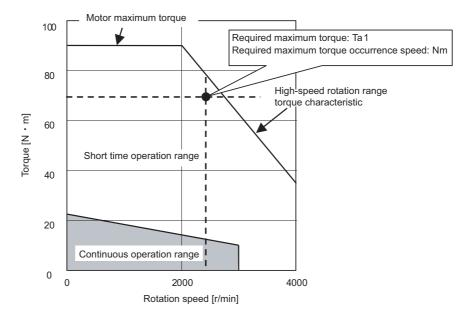
Motor torque characteristics
