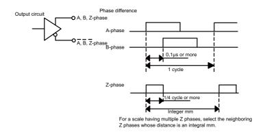
(Note) The above value is minimum value that can be received normally in the servo drive unit side.
