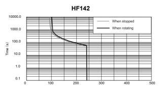
Motor current value (stall rated current value ratio %)
