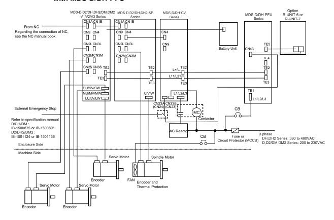
Appendix 4.3.3 MDS-D2/DH2-CV, D/D2-Vx/SPx, DH/DH2-Vx/SPx, DM/DM2-V3 Series with MDS-D/DH-PFU
