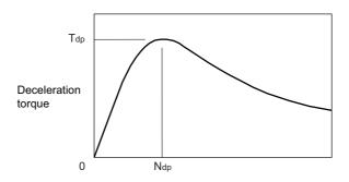
Deceleration torque characteristics of a dynamic brake
