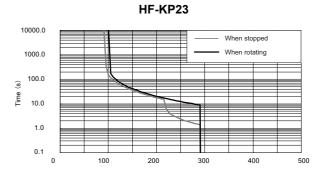
Motor current value (stall rated current value ratio %)
