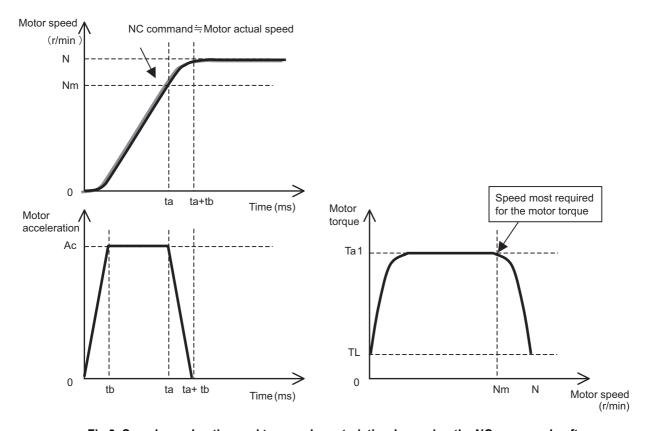
Fig 3. Speed, acceleration and torque characteristic when using the NC command soft acceleration/deceleration pattern + feed forward control
