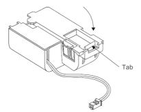
Close the cover by pushing until it is fixed with the tab of the locking part.
