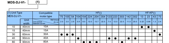
Indicates the compatible motor for each servo drive unit.
