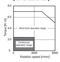
(Note) The solid line of short time operation range shows the characteristics of 3-phase 200V input.
