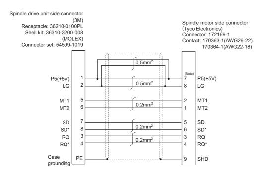
(Note) For the pin "7" or "8", use the contact "170364-1". For the other pins, use the contact "170363-1".
