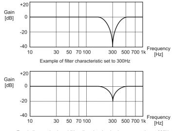
For shallow setting by additionally using the depth compensation at 300Hz
