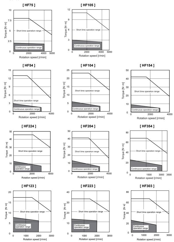
(Note) The solid line of short time operation range shows the characteristics of 3-phase 200V input.
