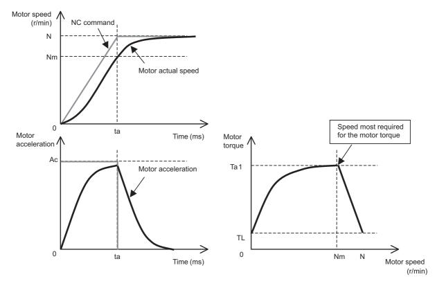
Fig.1 Speed, acceleration and torque characteristics when using the NC command linear acceleration/deceleration pattern + servo standard position control
