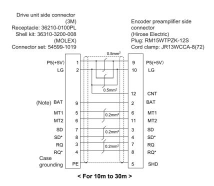
(Note) The above wiring diagrams apply to both MBA405W and MBE405W.
