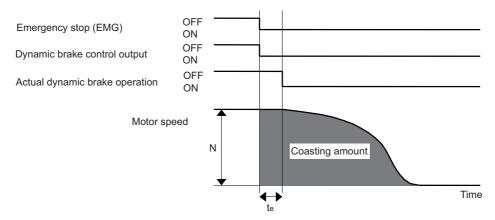
Dynamic brake braking diagram
